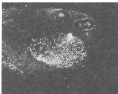
FIG. 2— Photograph of fingerprint on white paper after two weeks baking at 75°C followed by soaking for 5 min under running water.
